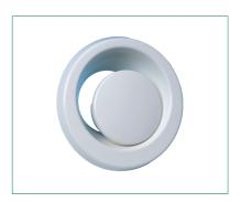
The KGEB exhaust valve is suitable for use in mechanical ventilation systems. The valve can be wall mounted or ceiling mounted and its air flow is simple to adjust. The KGEB has a low noise level, even if the pressure drop is high, and it has good natural sound attenuation.
